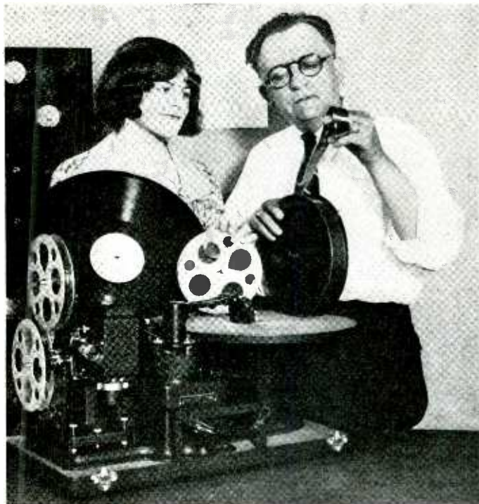
H. A. DeVry, vice-president of the QRS-DeVry Corporation, illustrates the comparative size of the standard film, for theater use, and of the 16 mm. film (left) used by most home projectors.
